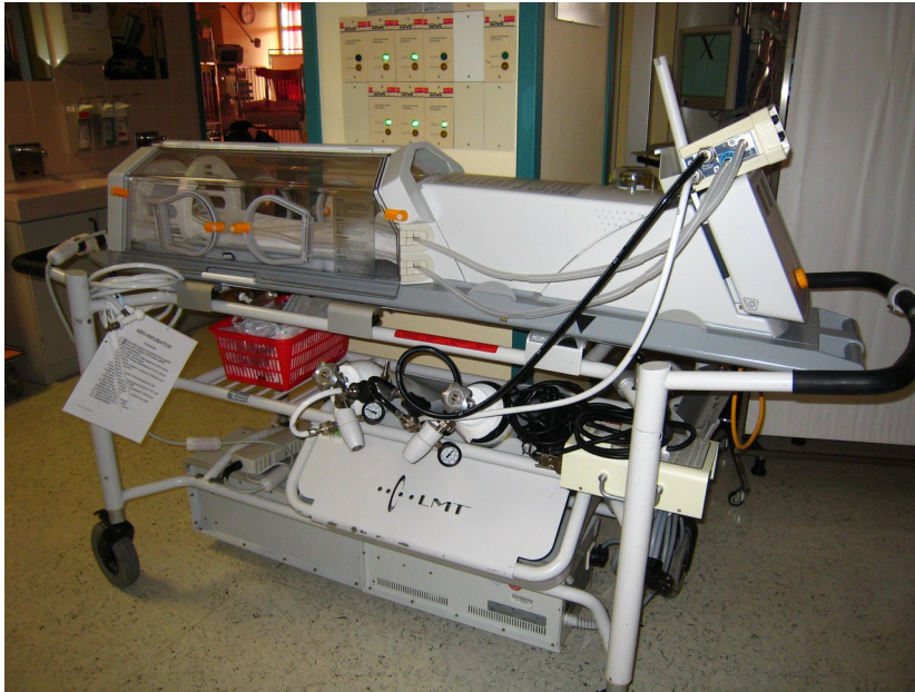
Figure 5.2.2. MRI Compatible Incubator used in our study. Ventilator and built in head coil are important part of the system.
