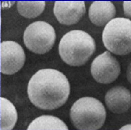
Electron microphotograph of spherical and irregular silica particles. [W.R.Melander, C.Horvath,
