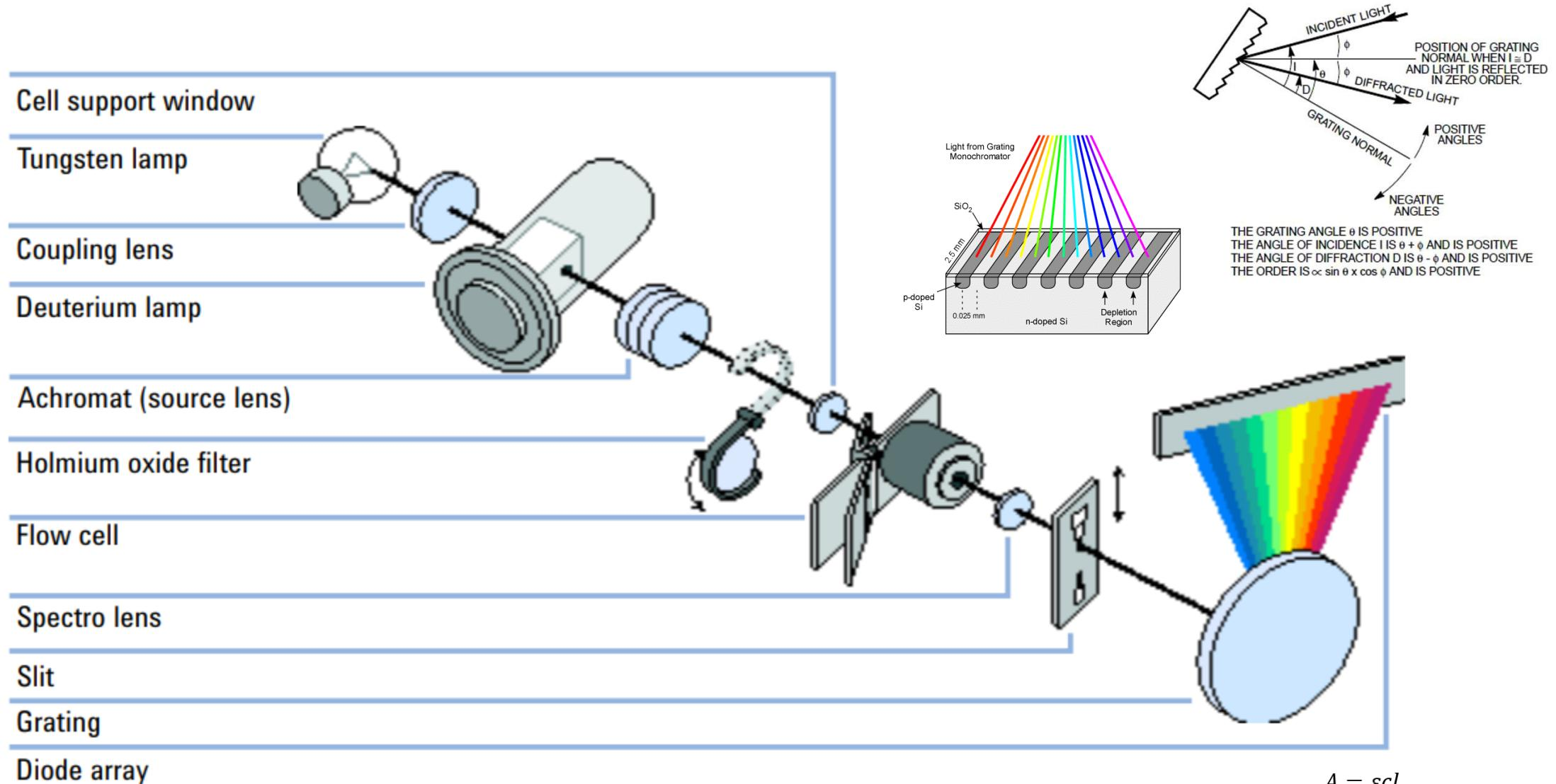
**Figure 3** Optical System of the Detector
