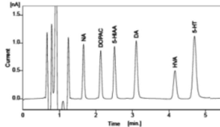
A sample is introduced in HPLC and separated on the chromatographic column. The column is connected to an ECD cell, an electrochemical sensor where a reaction takes place at an electrode. Electrochemically active substances that elute from the column undergo an electrochemical reaction, electrons are transferred resulting in an electrical current.
