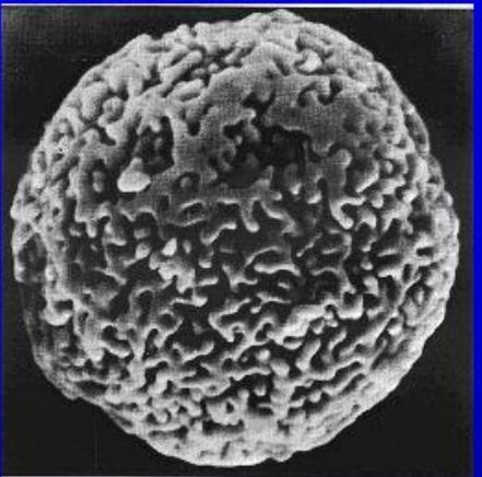
Macroporous spherical silica particle. [K.K.Unger,
