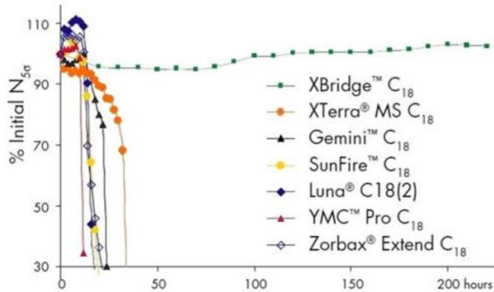
**Figure 1.** Stationary phase stability: efficiency loss as a function of time of purge with an aggressive mobile phase (analyte: acenaphthene; mobile phase: triethylamine, pH 10; 50 mM at 50°C). Figure reprinted with permission from reference (16).
