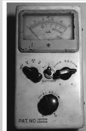
Fig. 2. Simple d.c. ohmmeter for measuring the length of the root canal using direct electric current
