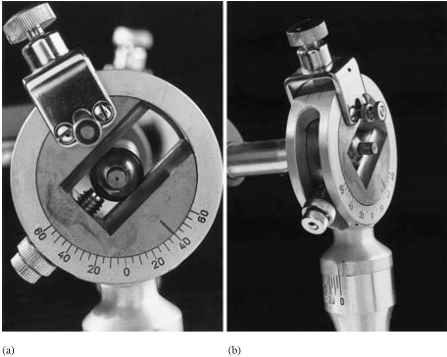
Fig. 11.15 (a) The condylar angle – the angle of the condylar track to the horizontal plane. (b) The Bennett angle – the angle of the condylar track to the sagittal plane.
