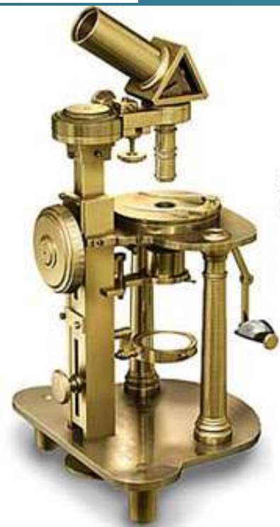
Cuff-style microscopes, popular in the mid-1700s, were the first to provide ease of use and accurate focusing mechanisms.
