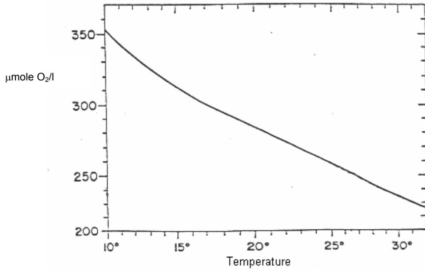
Fig.2. Oxygen content of air-saturated water versus temperature.
