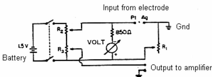
**Fig.1.** Scheme of the polarizing voltage and sensitivity control of an oxygen electrode. The variable resistor  $R_1$  is sensitivity control,  $R_2$  supplies a polarizing voltage of 0.6 V,  $R_3$  is for zero offset control.
